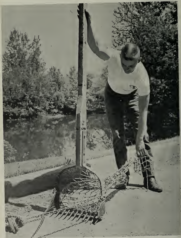
Fig. 7.—The dredge used in the Illinois River in the 1966 mussel survey. Photo by W. D. Zehr.
