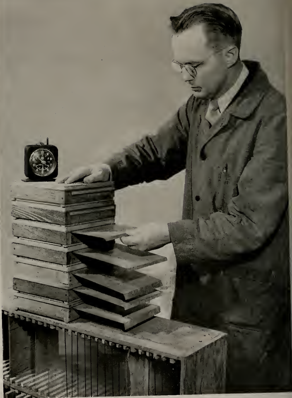
Exposure of flies to surfaces treated with insecticides is quickly accomplished with the cages shown here. The cages are inverted and stacked, with a treated panel on each cage; then the sliding metal panel in each cage is withdrawn to allow flies in the cage to have direct contact with the treated panel.
