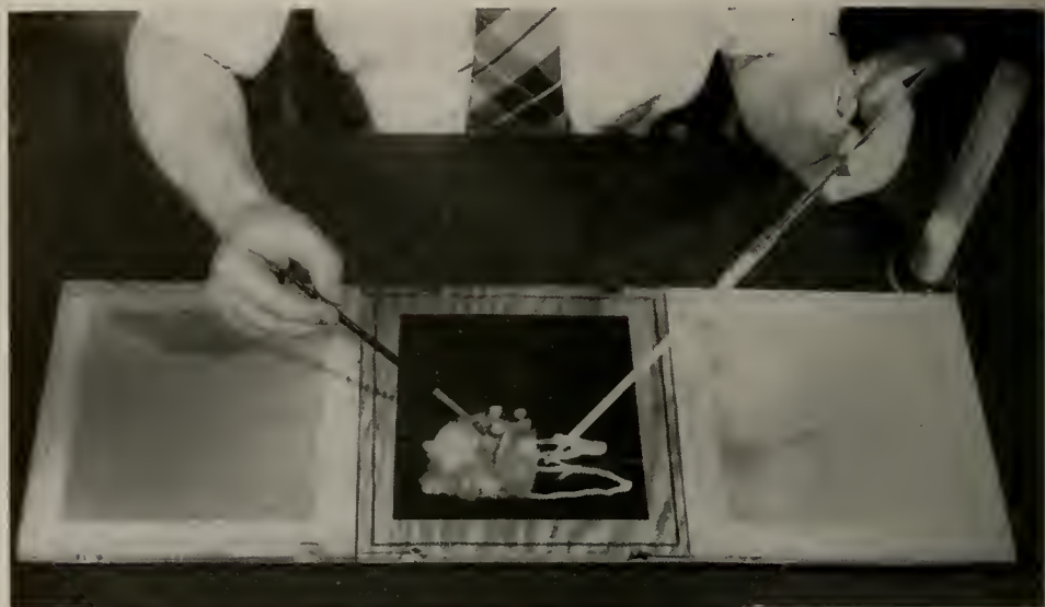
Fig. 4.—Three glass panels similar to those used in experiment. Left, panel with insecticide applied in settling spray tower; center, panel with insecticide being applied by means of brush and pipette; right, panel with insecticide already applied by means of brush and pipette.
