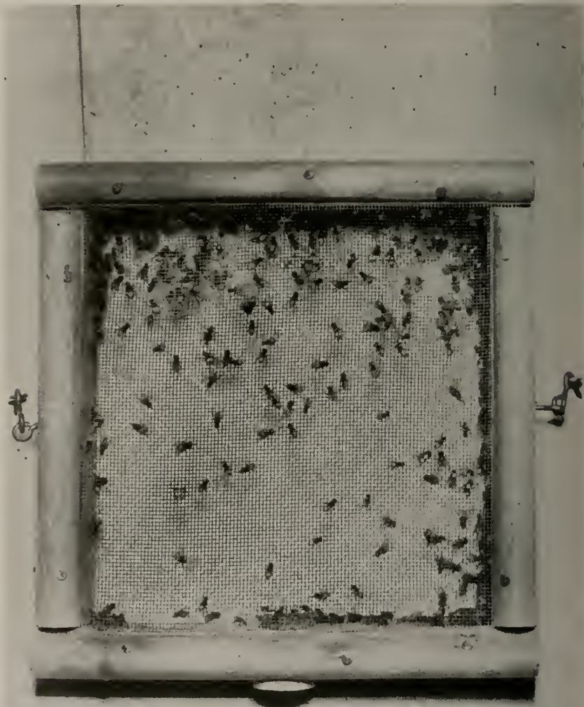
Fig. 2.—Practical method (not used in the experiments) of testing the toxicity of wall surfaces treated with residual insecticides. The exposure cage is hooked to the treated wall, and the metal panel is withdrawn to give flies in the cage direct contact with the wall for a given period of time.
