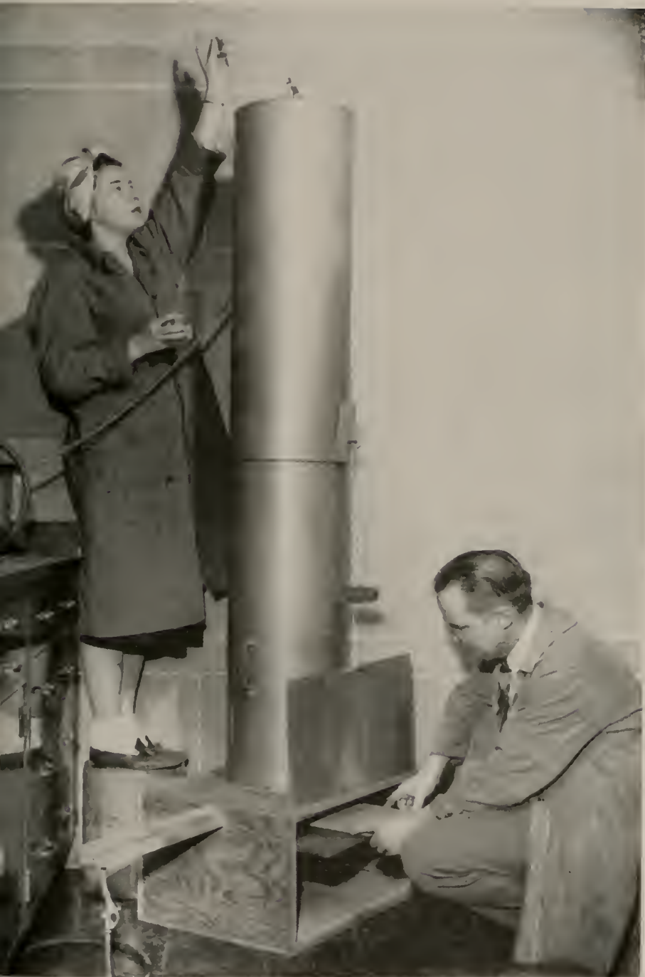
Fig. 5.—Settling spray tower. Insecticide is introduced by a pipette into the atomizer at top settling spray tower. A panel is placed on a sliding shelf in the bottom of tower. At 12.5 lbs air pressure, and after 3 minutes are allowed for settling, the dosage per square foot of shelf is approximately 32.4 per cent of the quantity placed in the atomizer.
