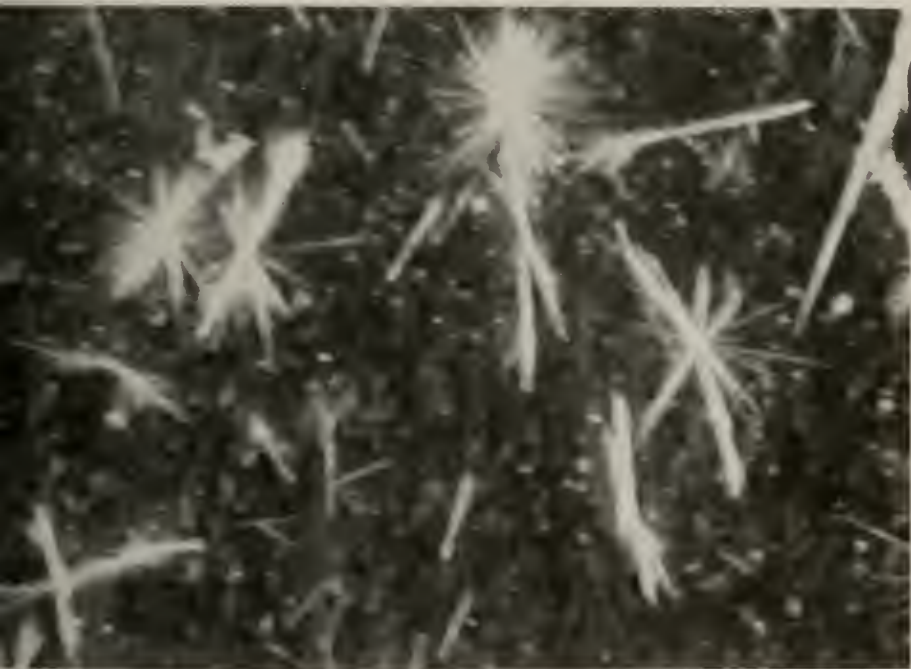
Fig. 7.—DDT crystallization from no. 9 oil on glass. \times 40 . The large crystals are plainly visible to the unaided eye.
