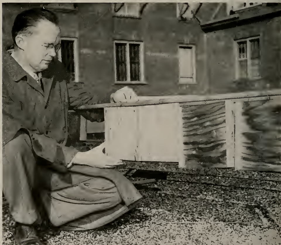
Fig. 14.—Securing treated panels to pipe rack for determining the effects of weathering upon toxicities of residues.
