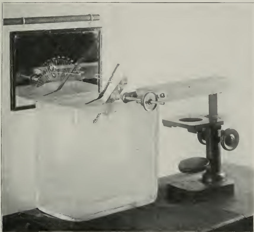
FIG. 3. APPARATUS USED IN MAKING ANGLE-OF-CONTACT MEASUREMENTS.
